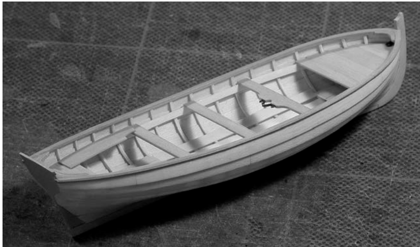
Gunwale, breast hook and transom knees completed
